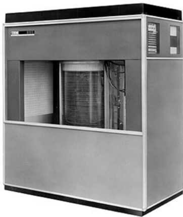
First disk storage unit by IBM (1956) Capacity: 5 megabytes Size: Refrigerator
